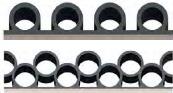
Pic. 3. Pipe wall profiles made using Krah technology
