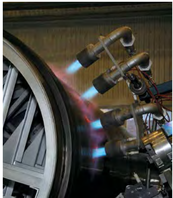
Pic. 6. Manufacturing of spiral wound PE pipe using Krah technology
