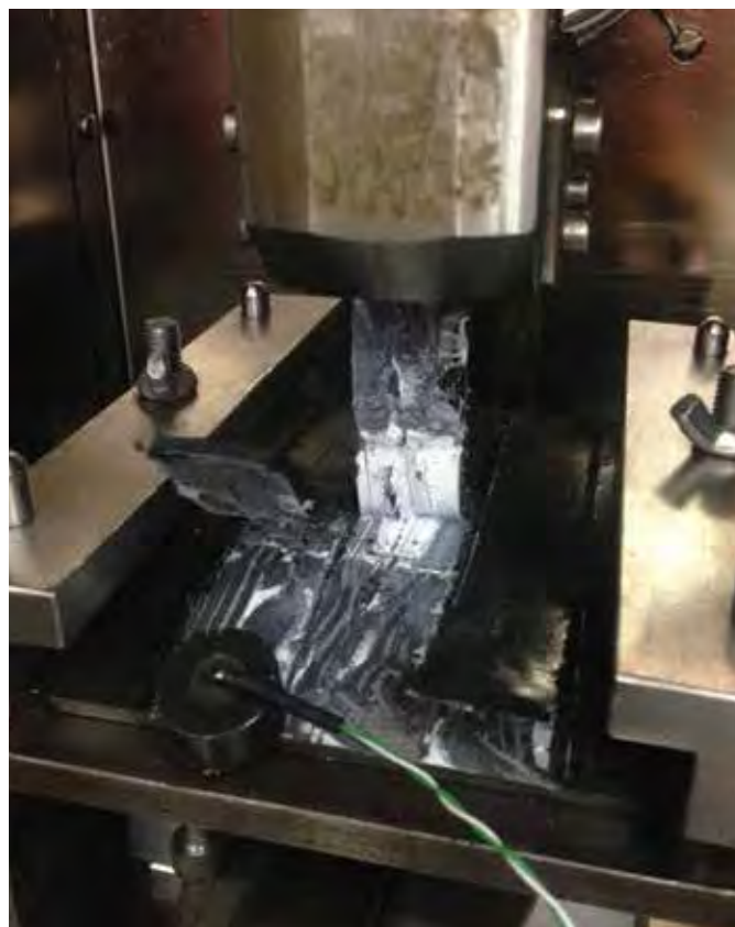
Pic. 2. Peel testing. Cohesive peeling of Armobond PE-2K
