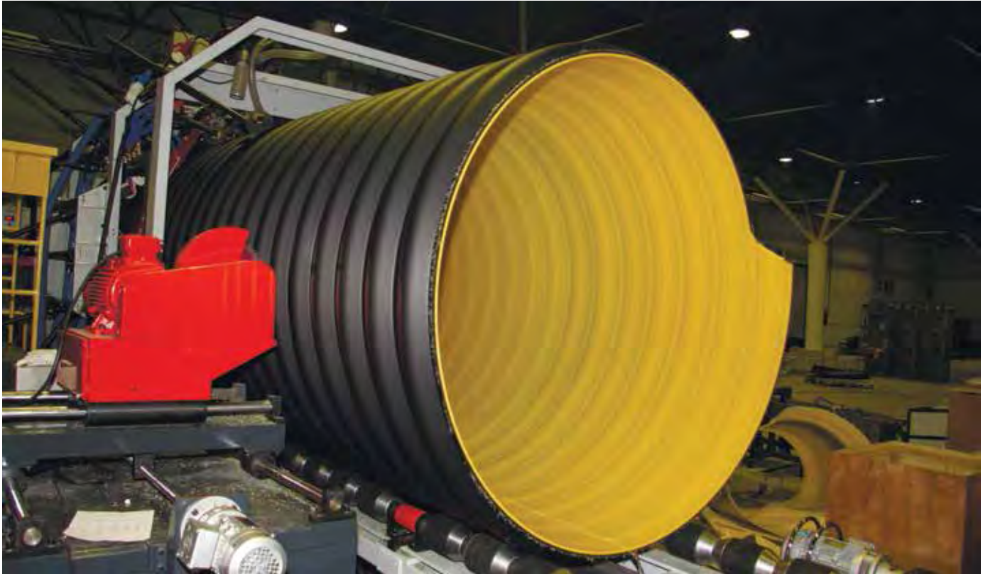
Pic. 5. Manufacturing of spiral wound PE steel reinforced pipe
