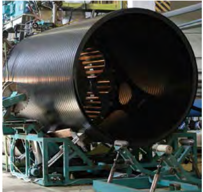
Pic. 1. Production of spiral-wound PE pipe with rectangular section profile
