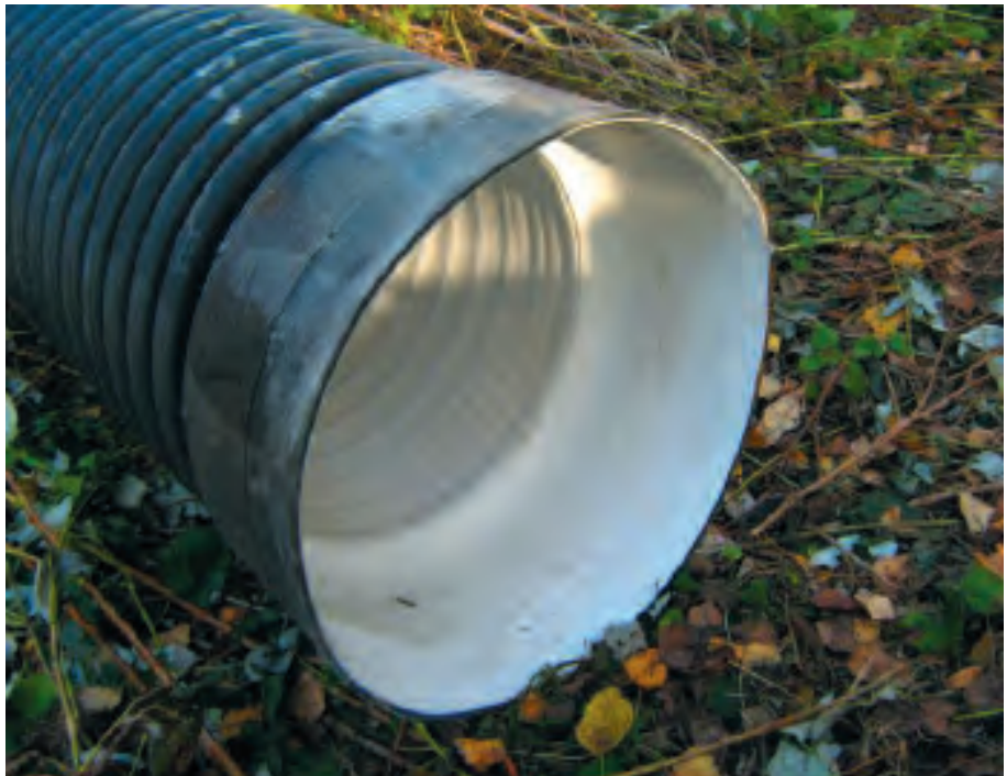
Molded joints often get deformation during improper transportation and storage
