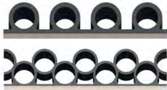
**Pic. 4. Profile of the spiral-wound pipe with steel reinforcement**
