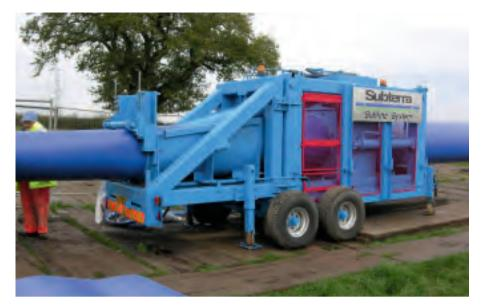
shape. It is then held in place by PP or PETP strapping. Once installed, the folded liner is pressurised to snap the strapping. The liner reverts to its original size and forms a close-fit within the host pipe. The pipe-forming unit is positioned near the manhole. Long length installation up to 1 km in a single insertion is possible. Standard length is from 200 to 300 metres.
